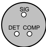
Typical Pellistor Pinout
