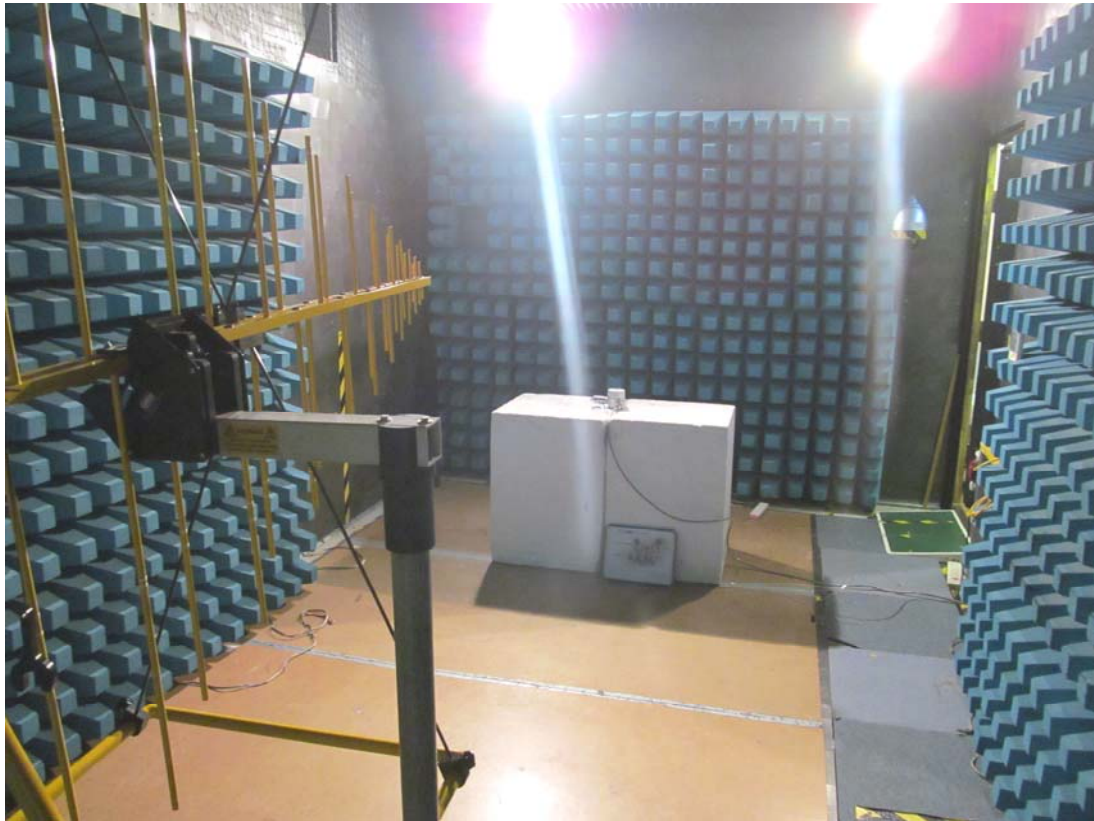
Photograph 5.4.1 Radiated emissions testing, chamber
