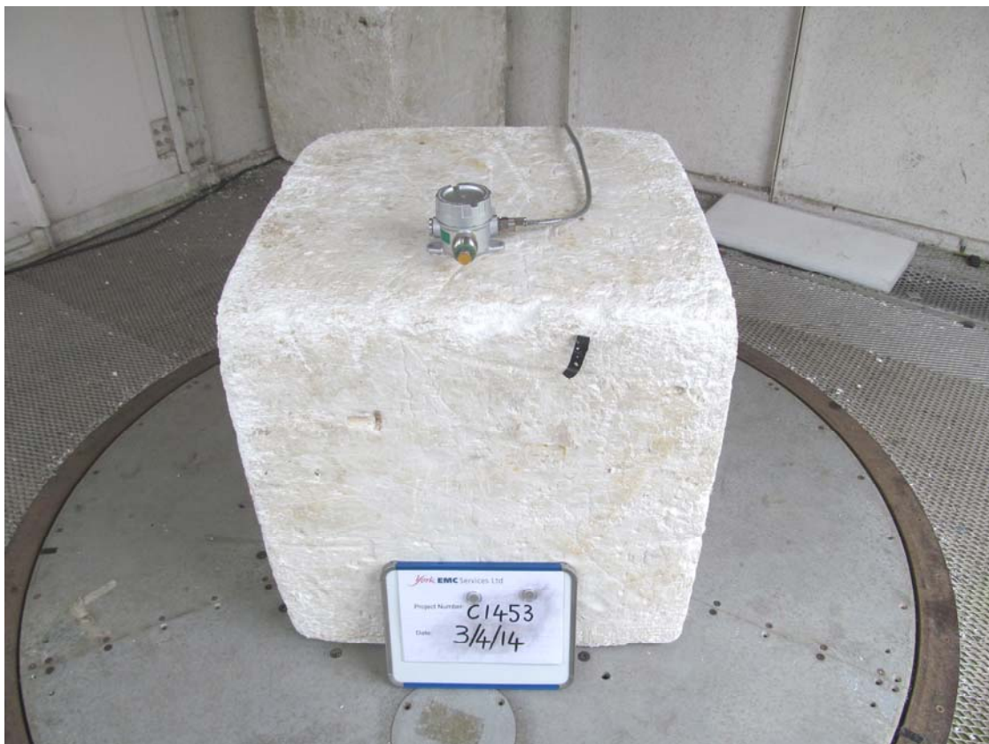
Photograph 5.4.3 Radiated immunity > 1GHz testing
