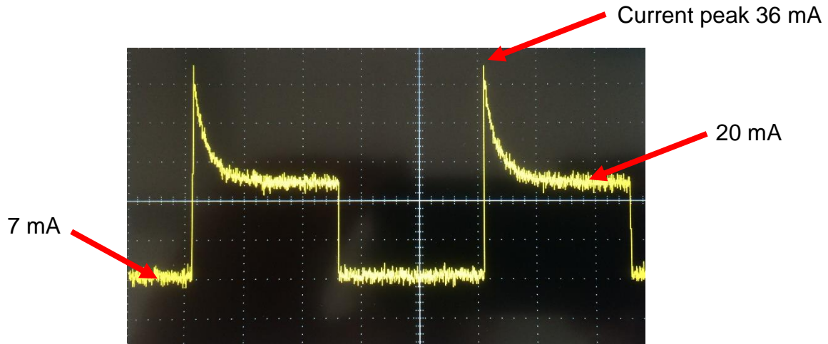
Current waveform for Premier low power sensor.
