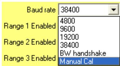
The Serial Tx and Rx pins will only be changed to calibration pins when the sensor has been powered for approximately 10 minutes. This makes sure that the user cannot be calibrated before the sensor has been powered for a sufficient time.
