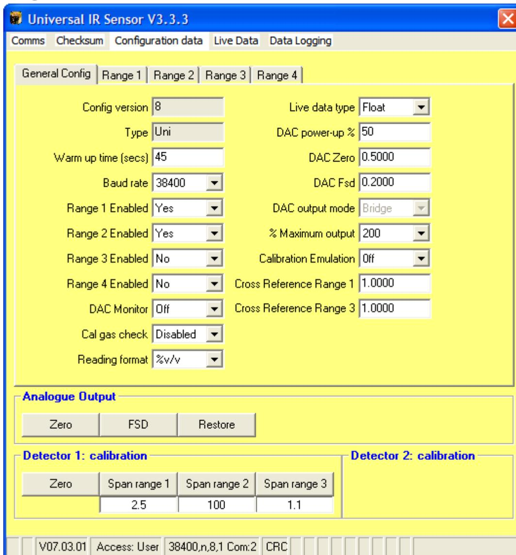
Note 1: The sensor is fitted with a DAC, as such the Analogue output buttons are available.
