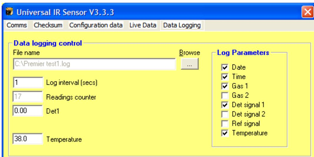
Note the readings counter incrementing every reading.
