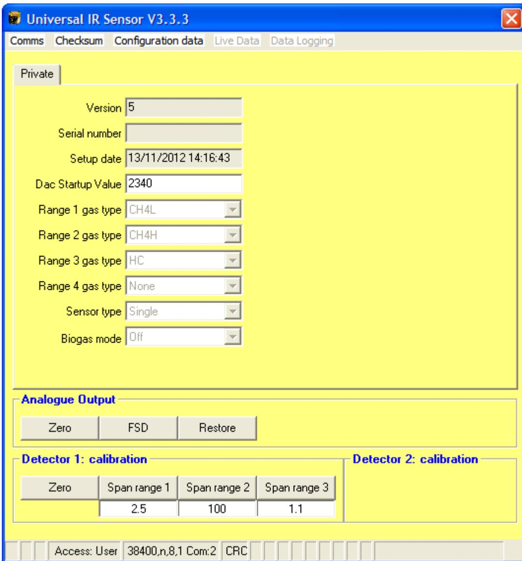
The only field that can be changed by the user is the *Dac Start-up Value*. All the remaining fields are setup during manufacture and cannot be changed by the user.
