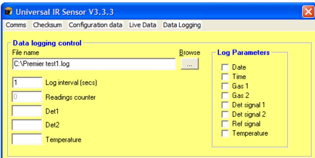
Enter a file name, with the .log extension, or use the *Browse* button to locate an existing file. If an existing file is selected then it will be over-written and all data will be lost. Set the log interval to the desired frequency.
